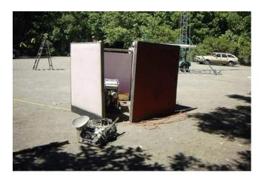
SCCARA's AC generator surrounded by cubicle walls to reduce engine noise. This generator and several DC car batteries supported power needs, SCCARA stations were all based on "emergency power."
